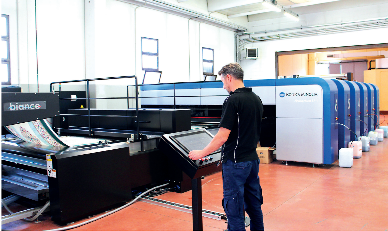
Above: Nassenger SP-1, an ultra-high-speed inkjet textile printer that uses a single-pass system
