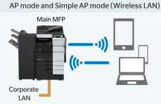
Up to 5 devices can access bizhub 658e/558e/458e simultaneously in AP mode with UK-212 equipped. Up to 4 devices can access bizhub 658e/558e/458e simultaneously in Simple AP mode with UK-215.
