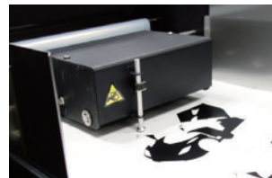
Air-suction paper feeding for minimum damage to the paper.
