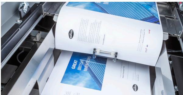
Collating station with the "tumbler" mechanism prepares the book for stapling and folding
