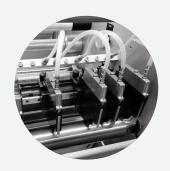
**GM SmartCrush** - An ultra-quick set knives system, allowing fast and precise setting of each crush knife – also while running.
