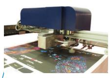
NEW PALLET FEEDER New pallet feeder featuring easy paper loading and new feeding suction system for 75x120 cm (29x47'') sheets.
