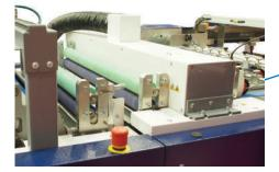
NEW CORONA MODULE In-line system made to optimise varnish adhesion on complex printed substrates
