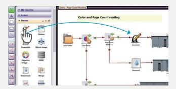
The operator can use icons to easily create a pre-press workflow. Conditional branching depending on the file content, additions or changes to details of processing, and setting of which printer to use are all easy to configure.
