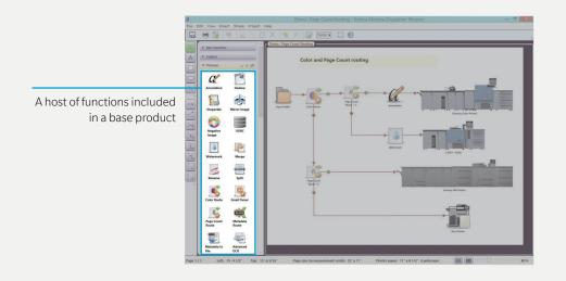
The basic AccurioPro Connect product includes a workflow builder, a preflight function, an imposition function, and a host of other nodes to support workflow automation.
