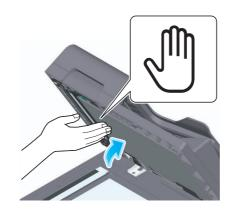
→ Press the Hand mark in the center of the **Opening and Closing Guide**, and check that the **Opening and Closing Guide** is locked securely.
